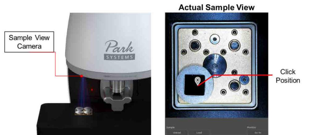
Figure 13. Sample navigation is made much easier by default off-axis sample view camera and fast moving XY stage. The picture on the left indicates the physical location of the camera while the right picture depicts an actual screen shot.
