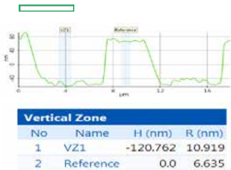
Figure 2a. AFM topography image of measurement site #1 with green inset rectangle denoting specific area of interest. This area's line profile is also provided along with recorded step height (H) and roughness (R) values gathered by measuring sites VZ1 (in the first device pit) and Reference (in the raised area between the first and second device pits).
