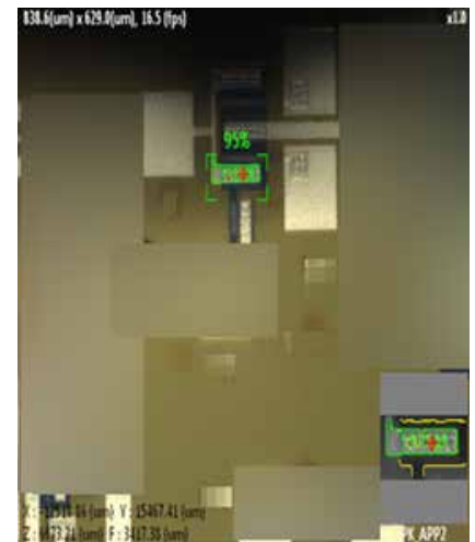
Figure 1b. Optical camera feed from the XEA software interface displaying a 95% confidence level in the software's ability to recognize the sample pattern.
